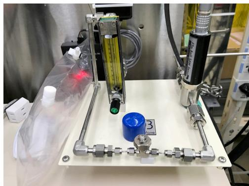
**Fig. 2** Experiment setup for injection of saturated moisture of a gas bad on the left into a pipe line close to ball SAW trace moisture sensor.[3]
