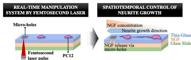
**Fig. 1.** Schematic diagram of real-time manipulation system to create femtosecond laser-fabricated micro-holes that release nerve growth factor (NGF) and induce neurite guidance.
