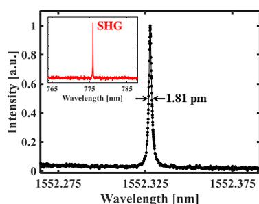
**Fig. 1.** Fundamental resonant spectrum of a SiC PC nanocavity. The inset shows the experimental SHG spectrum
