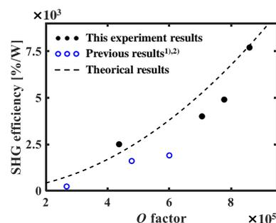
**Fig. 3.** SHG efficiency (circles) for  $Q$  factors including previous results<sup>1),2)</sup>. The dashed line indicates theoretical results.
