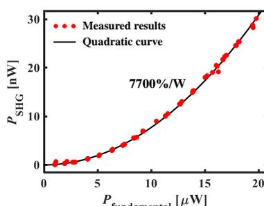
**Fig. 2.** Measured SHG power as a function of fundamental power in the nanocavity with  $Q = 8.6 \times 10^5$ .
