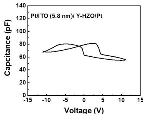
Fig. 3 C-V curve of Pt/ITO/Y-HZO MFS structure
