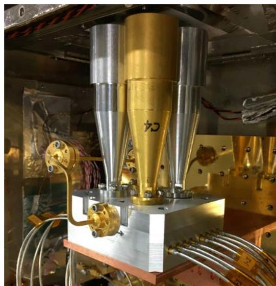
Fig. 1. Photo of the 4-beam mixer holder mounted inside cryostat. Signals of 2 mm wavelengths are coupled through four corrugated horns attached at the upper side. The single LO injection port is seen at the near-side of the block. IF/DC are conducted by using 16 coaxial cables.
