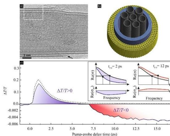
**Figure 1:** a) Atomic STEM ADF image of C@BN@MoS<sub>2</sub> NT heterostructure; b) model of C@BN@MoS<sub>2</sub> NT heterostructure; c) The switch from  $\Delta T/T > 0$  at early times to  $\Delta T/T < 0$ .
