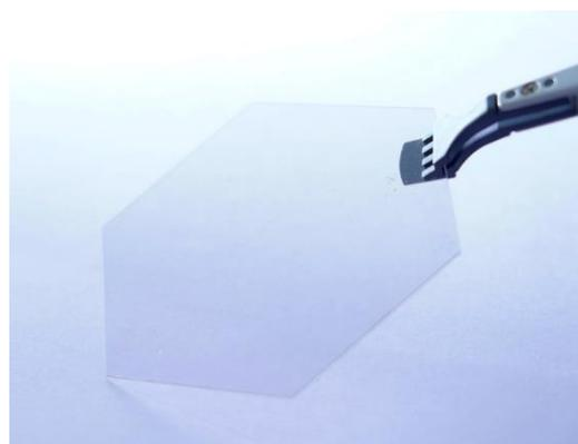
**Fig. 2** 2-inch GaN wafer grown with the new point seed method, showing high transparency because of the low oxygen concentration.
