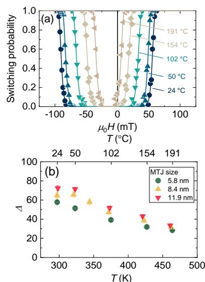
Fig. 1 (a) Switching probability measured under application of  $H_{\text{pulse}}$  with pulse duration of 1 s for  $D = 5.8$  nm at various temperatures. (b) Temperature dependence of  $\Delta$  for  $D = 5.8, 8.4,$  and  $11.9$  nm.
