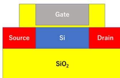
Fig.1 SOI MOSFET simulated
