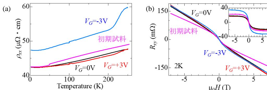
Fig.1 (a)Temperature dependence of resistivity of Pd/NFO
