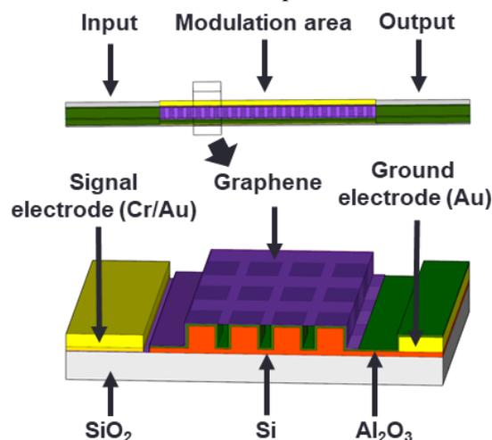
Fig. 1. Schematic structure of the graphene loaded silicon SW-MS BG.
