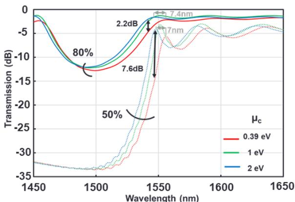
Fig. 2. Transmission spectra of the device with for various  $\mu_c$  at period count 20.
