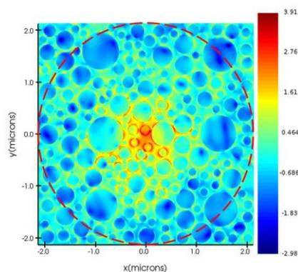
Fig. 2. Electric field intensity distribution for the top view of SERS with microsphere in log scale.
