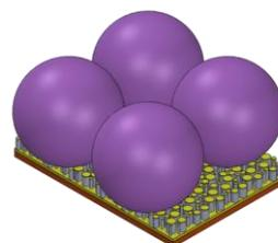
Fig. 1. Polystyrene microspheres coated on metal pillars SERS substrate
