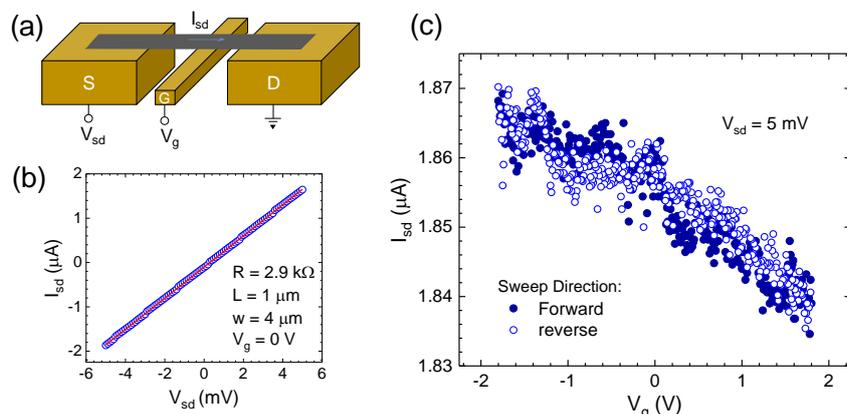
Fig. 1. (a) Schematic diagram of suspended GNR with local bottom-gate; (b) transport characteristic (at  $V_g = 0$  V) of a suspended ribbon (length ( $L$ ) = 1  $\mu\text{m}$ , width ( $w$ ) = 4  $\mu\text{m}$ ); (c) ambipolar characteristics of the ribbon.
