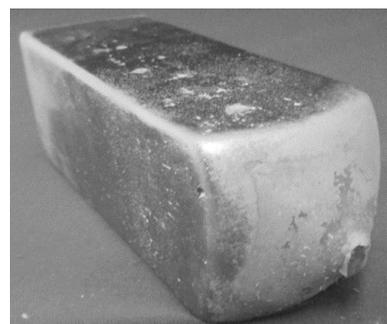
Fig.1 Photograph of 1.7"□ Fe-Ga grown crystal by VB method
