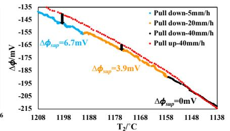
Fig.2  $\Delta\phi$  plotted a function of  $T_2$  with velocity change ( $-0.1$ mA).
