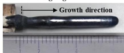
Fig. 2 LiCoO<sub>2</sub> single crystals grown at mirror tilting angle  $\theta = 10^\circ$ .
