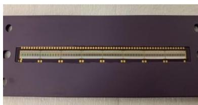
Fig2 Ceramic 64ch MPPC
