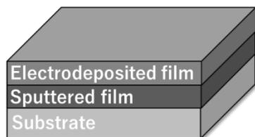
Fig. 1 Pattern diagram of laminated film.
