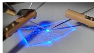
Fig. 3 Emission image of micro LED after transfer process
