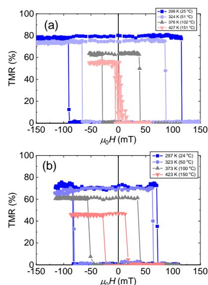
Fig. 1 Temperature dependence of  $R$ - $H$  curves for interfacial- ((a),  $D = 16.3$  nm) and shape-anisotropy MTJs ((b),  $D = 5.0$  nm).
