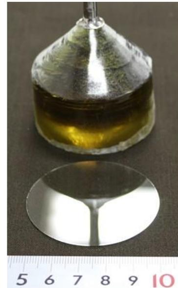
Fig. 1 VB grown 2"  $\phi$   $\beta$ -Ga<sub>2</sub>O<sub>3</sub> crystal ingot and polished wafer
