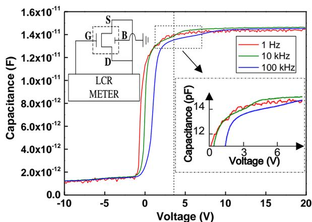
Fig. 1.  $C_{GC}$ - $V$  curve of NO10 sample.
