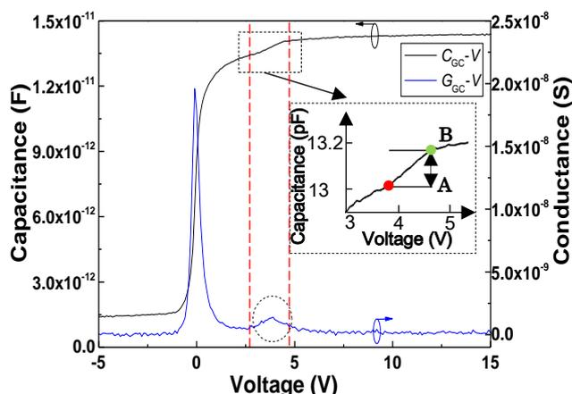
Fig. 2.  $C_{GC}$ - $V$  and  $G$ - $V$  curve of NO10 sample at 1 kHz
