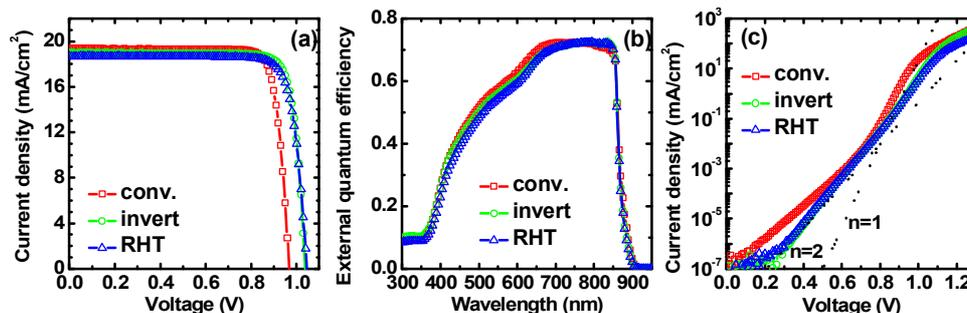
Fig. 1 (a) I-V characteristics, (b) EQE spectra and (c) dark I-V curves of high speed grown GaAs solar cells with various structures: conventional, inverted and rear hetero junction
