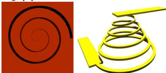
Figure 1: Schematics of the device layout, a chiral conical spiral. Left: a schematic of the resist surface after milling of the structure into the surface. Right: a schematic of a metal wire without the supporting PMMA.
