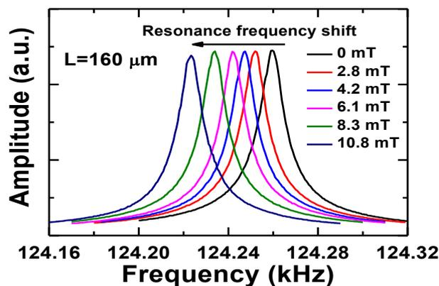
**Fig. 1** Resonance frequency response of the FeGa/SCD cantilever upon varying applied magnetic fields. The resonance frequency shifts to the lower frequency side with increasing the applying magnetic field.
