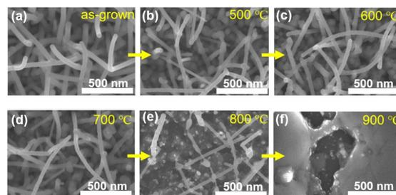
Figure1. SEM images of (a) as-grown i-Ge/p-Si core-shell NWs and after RTA annealing at (b) 500 °C, (c) 600 °C, (d) 700 °C, (e) 800 °C, (f) 900 °C with fixed annealing pressure of 100 Pa and annealing time of 1 min.
