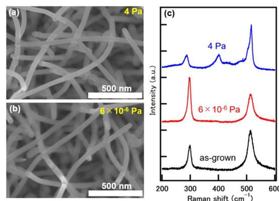
Figure2. The i-Ge/p-Si core-shell NWs under different pressure treatments; of (a) SEM images of NWs annealed under pressure of (a) 4 Pa, (b) SEM image of  $6 \times 10^{-6}$  Pa, and (c) their Raman spectra.
