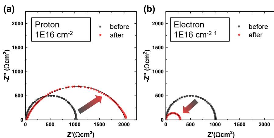
Figure 1. Nyquist plots for CIGS thin film solar cells before and after (a) proton (380keV,  $1E15 \text{ cm}^{-2}$ ) and (b) electron (2MeV,  $1E16 \text{ cm}^{-2}$ ) irradiation.
