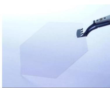
Fig. 2 2-inch GaN crystal grown by the advanced point seed technique. (after CMP process)
