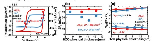
Fig. 2: (a) P-V and I-V curves of stacks with Al<sub>2</sub>O<sub>3</sub> and SiO<sub>x</sub> IL of 11.2-nm-thick HZO. (b) 2P<sub>r</sub> and (c) V<sub>c</sub> as a function of HZO thickness for devices with Al<sub>2</sub>O<sub>3</sub> and SiO<sub>x</sub> IL.
