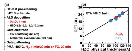
Fig. 1: (a) Key process steps for fabricating the devices used in this work. (b) CET as a function of physical thickness of HZO for stacks with Al<sub>2</sub>O<sub>3</sub> and unintentional SiO<sub>x</sub> IL.
