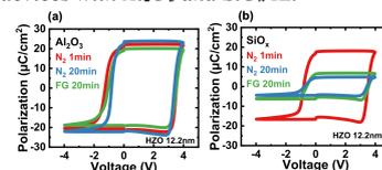
Fig. 3: P-V and I-V relationships after annealing for devices with (a) Al<sub>2</sub>O<sub>3</sub> and (b) SiO<sub>x</sub> IL at the HZO thickness of 12.2-nm.
