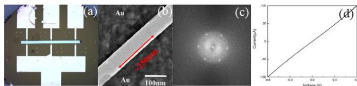
Fig 1. (a) The fabricated GNR device, (b) TEM image of suspended GNR, its width is indicated by red arrow, (c) The corresponding FFT pattern in (b), (d) I-V curve of wide GNR in (b).
