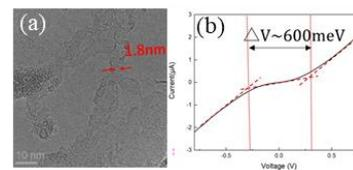
Fig 2. (a) TEM image of the fabricated narrow GNR with a width of 1.8 nm. (b) I-V curve of narrow GNR in (a).
