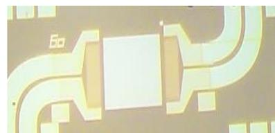
Figure 1: SAW device.
