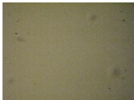
Fig.2 Surface condition of InP/Si substrate observed by Nomarski microscope
