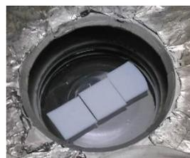
Figure 2 Alignment of PTFE tips on a SiO<sub>2</sub> target
