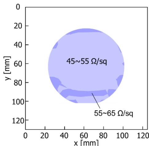
Fig. 1 Distribution of the sheet resistivity in the 4-inch substrate.
