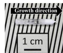
Figure 1 (Ce<sub>0.015</sub>La<sub>0.600</sub>Y<sub>0.385</sub>)<sub>2</sub>Si<sub>2</sub>O<sub>7</sub> crystal grown by micro-pulling-down method.
