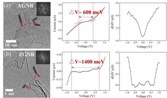
Fig 2. Images of an ultra-narrow AGNR (a) and ZGNR (b) and their electrical conductance
