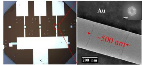
Fig. 1: The fabricated GNR device.
