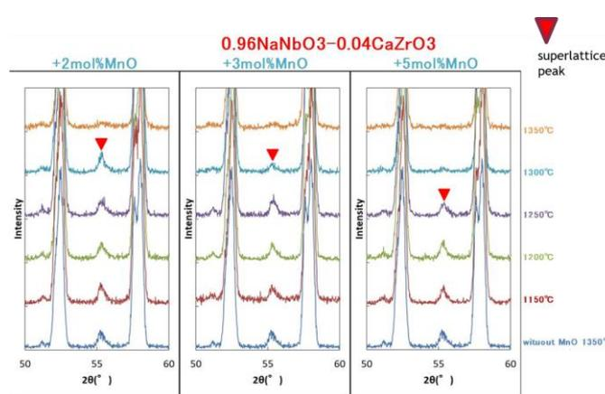
Fig. 1. XRD patterns of  $0.96\text{NaNbO}_3\text{-}0.04\text{CaZrO}_3$  ceramics sintered at  $1100\text{-}1350^\circ\text{C}$ .
