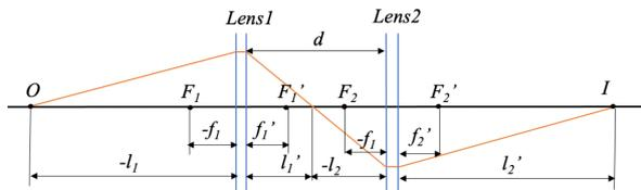
Fig. 2. Optical path of double lenses system.
