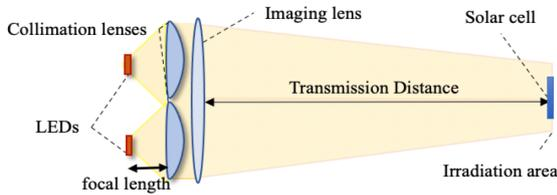
Fig. 1. The collimation scheme of multi-LED OWPT system.
