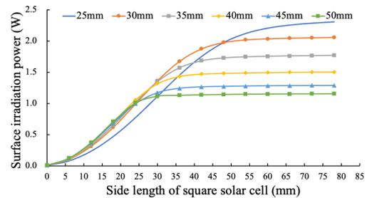
Fig. 3. Simulated irradiation power at 1 m with different focal length of collimation lens.
