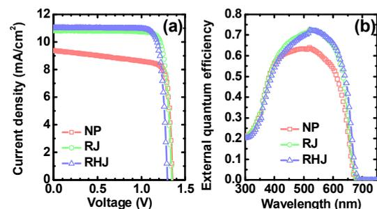
Fig. 1 (a) I-V characteristics under AM1.5G and (b) EQE spectrum of InGaP solar cells with different device structures
