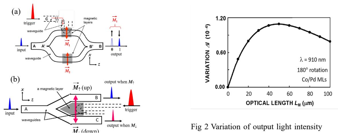
Fig. 1 (a) MZI- and (b) splitter-type memory cells.
