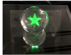
Fig. 2 Principle of imaging an aerial image with two clear spheres.
