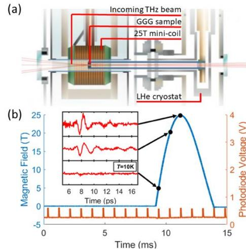
**Fig. 1.** (a) RAMBO system. The sample is mounted on a sapphire rod, connected to the cold finger of a liquid helium cryostat. The 25-T mini-coil magnet is immersed in liquid nitrogen. (b) Magnetic field pulse (blue), and time-domain THz waveforms (red) recorded at three magnetic fields within the magnetic field pulse.
