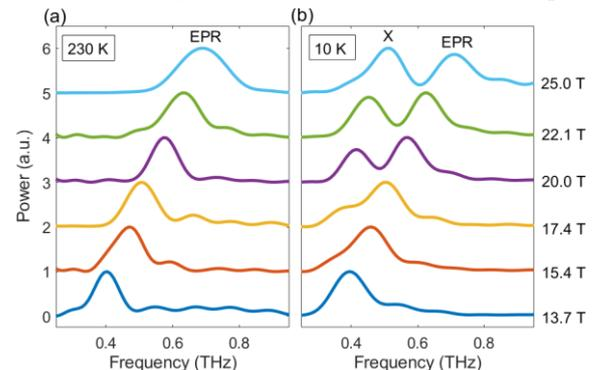
**Fig. 2.** Power spectra of THz radiation transmitted through the GGG crystal at (a) 230 K and (b) 10 K at various magnetic fields. Curves are vertically offset for clarity.
