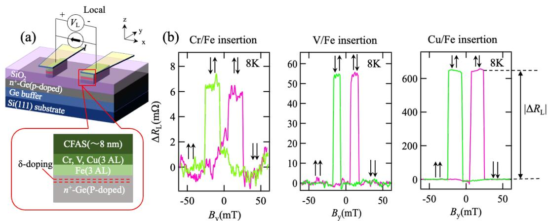
Fig. 1(a) Schematic of the fabricated LSV devices with NM insertion at the CFAS/Ge interfaces. (b) Two-terminal local spin signals measured at 8K for LSV devices with Cr/Fe, V/Fe, and Cu/Fe insertion layers.
