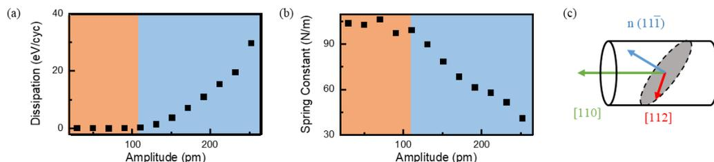
Fig. 2: (a) From the dissipation of the LER, the deformation of Au NC could be divided into elastic deformation (orange) and plastic deformation (blue). (b) The spring constant of the NC. (c) An illustration of slip system for  $\langle 110 \rangle$  NCs.
