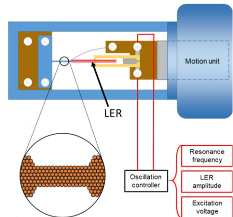
Fig. 1: Schematic illustration of the home-made TEM. The Au NC was suspended between the edge of the LER and a counter plate. The LER was managed by an oscillation controller.
