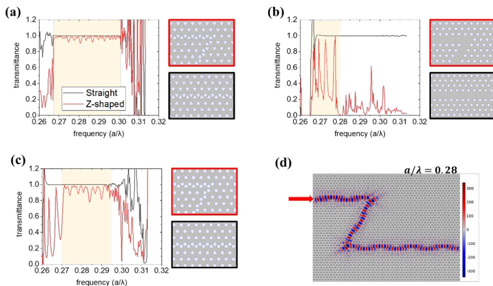
Fig.1 Calculated transmittance spectra of (a) bearded interface VPhCWGs, (b) W1WGs and (c) bearded interface TPhCWGs, red for Z-shaped waveguides and black for straight waveguides. (d) The out-of-plane magnetic field component of light traveling through the Z-shaped TPhCWG in (c), at the frequency  $a/\lambda = 0.28$ .
