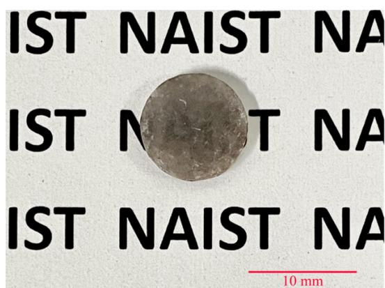
Figure 1 Photograph of the Au-doped CsCl translucent ceramic specimen.
