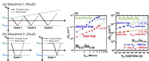
Fig. 1 (a) Cycle measurement with same  $V_{stop}$  and increasing  $V_{start}$ . (b) Hold time measurement with same  $V_{stop}$  and  $V_{start}$ . The hold time is varied from 1, 10, 100 and 999s, respectively.
