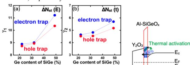
Fig. 3 Acceleration factor (a)  $\gamma_1$  and (b)  $\gamma_2$  as a function of Ge content of SiGe.
