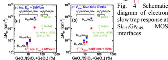
Fig. 5 (a) Hole and electron  $\Delta N_{st}$  at  $E_{ox}$  of 6MV/cm and (b) Hole and electron  $\Delta N_{st}$  when hold time is 999s as a function of percentage of GeO<sub>x</sub> in SiGeO<sub>x</sub>.
