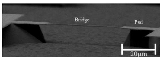
Fig. 2 A SEM image of the  $\langle 111 \rangle$  strained Ge microbridge
