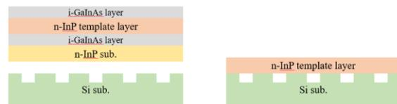
Fig.1 Schematic of InP/Si substrate using gas out channel
