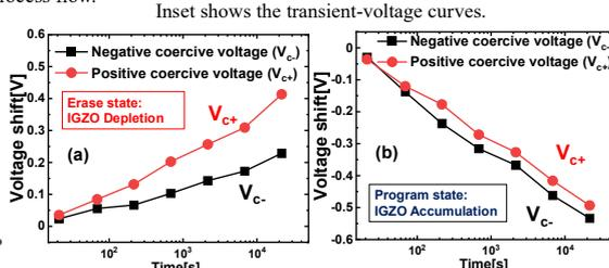
Fig. 5. Extracted shift of V<sub>c</sub> in erase (a) and program (b) state. Red and black show positive V<sub>c</sub> (V<sub>c+</sub>) and negative V<sub>c</sub> (V<sub>c-</sub>), respectively.
