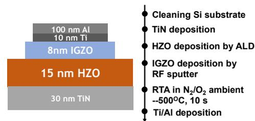
Fig. 1. Schematic illustration of the device structure of TiN/HZO/IGZO/Ti and the fabrication process flow.
