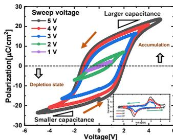
Fig. 2. P-V curves with different sweep voltage. Inset shows the transient-voltage curves.
