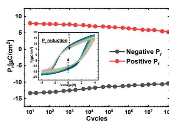
Fig. 3. Endurance characteristic of the fabricated capacitor. Up to 10<sup>8</sup> cycles program/erase is achieved.
