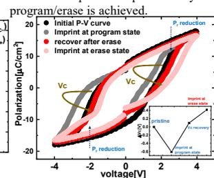
Fig. 6. Measured P-V curves with different device state. The inset is the extracted V<sub>c</sub>.
